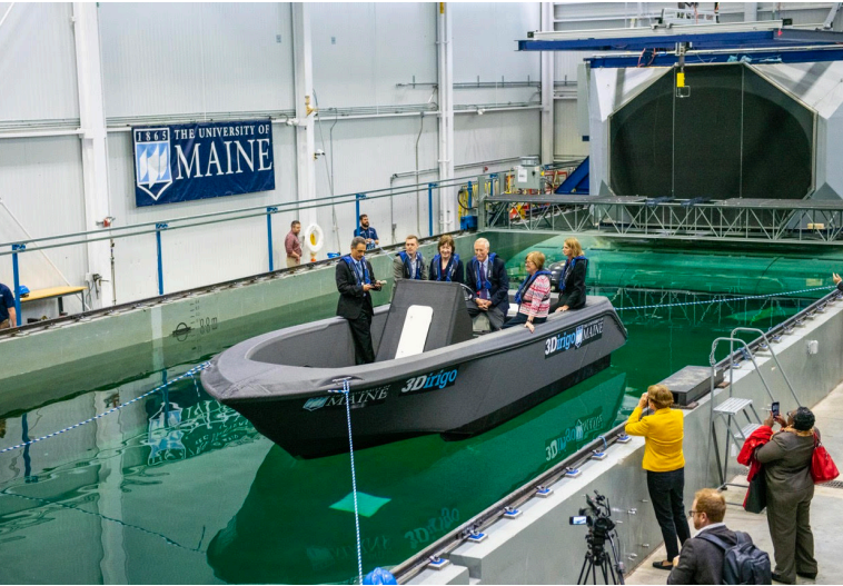
The 3Dirigo was produced by the world's largest 3D printer within 72 hours
